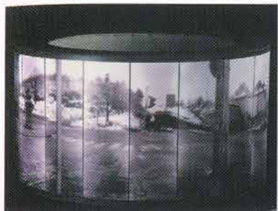
Henger camera obscura Δ Ø 80 cm, m=43 cm Δ Cylinder camera obscura
